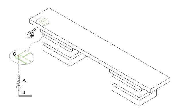
• Hand tighten the bolts with the Allen key and make sure the bench top is well secured to each support bracket and each pedestal base.
