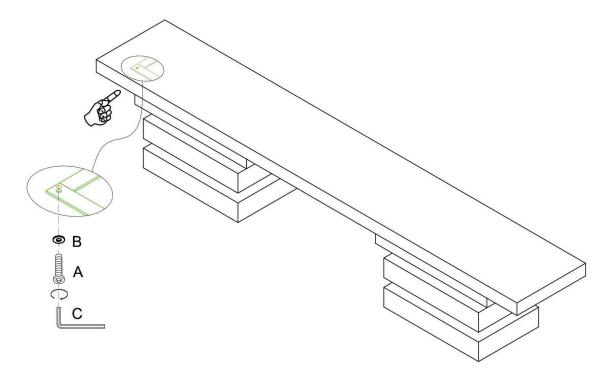
d) Hand tighten the bolts with the Allen Key and make sure the Bench Top is well secured to each assembly bracket and each Bench Pedestal base.
